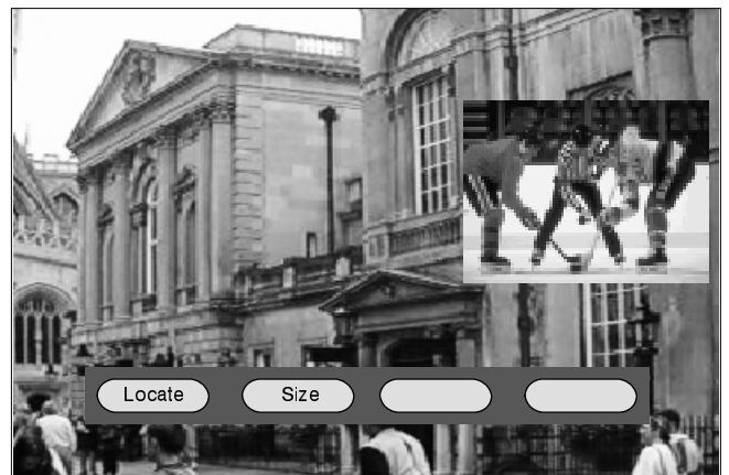
The PIP picture has been moved to an alternative position and made smaller by pressing the red key followed by the green key.
